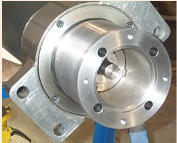
Engine not mounted, only engine flange and drive pinion are visible.
